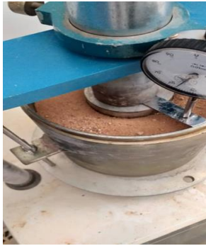
Fig. 1. Setup of Circular Footing
